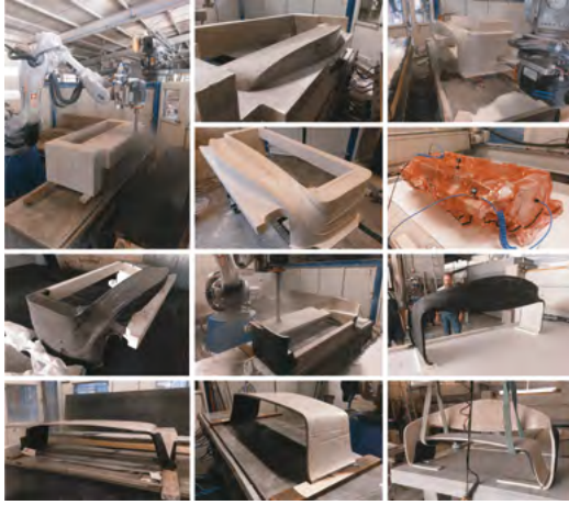
01 Fabrication process of Möbius Sofa (Photos by Generelli SA, 2016)
